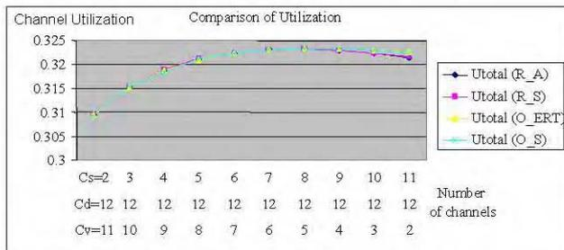
Fig. 7 Channel Utilization under Channel Distribution of Servers
