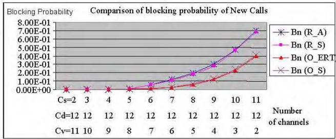
Fig. 3 Blocking Probability of New Calls under Channel Distribution of Servers.
