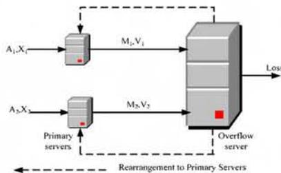
Fig. 2 Overflow system model in two traffic streams with rearrangement
