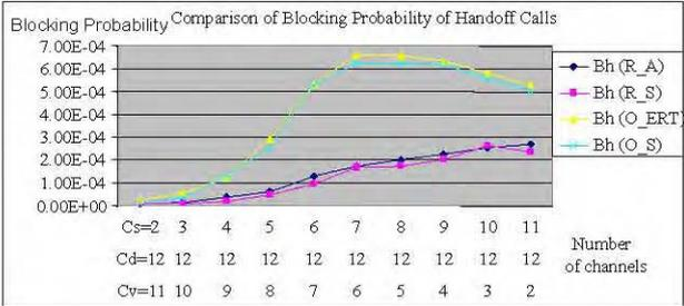
Fig. 4 Blocking Probability of Handoff Calls under Channel Distribution of Servers
