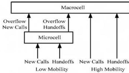
Fig. 1 Overflow system with primary cells
