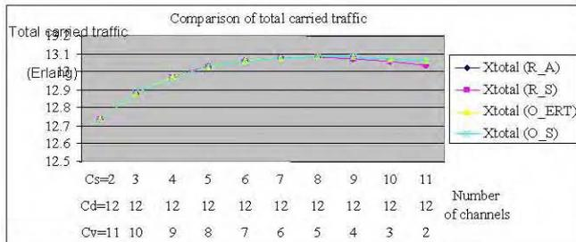
Fig. 6 Total Carried Traffic under Channel Distribution of Servers
